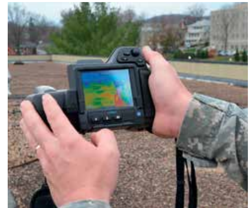
The infrared camera is used to assess the roof of Cameron Hall. – VMI Photo by Kelly Nye.
